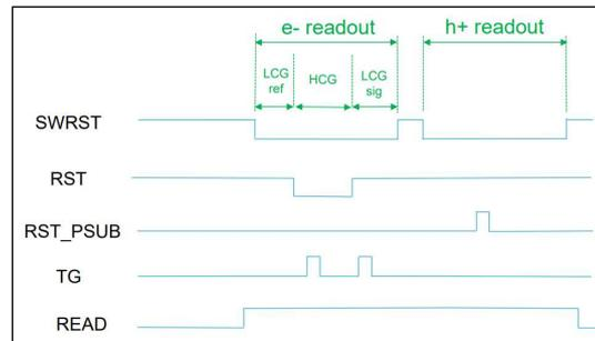
To make use of electrons and holes, the quantum efficiency for both NEEDS TO BE EQUAL !!! This is only possible if the collection volume is fully isolated.
