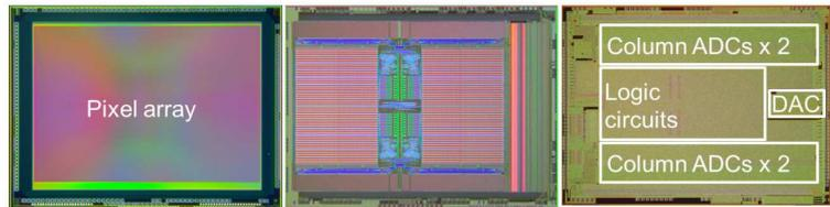
A micrograph of top layer    A micrograph of middle layer    A micrograph of bottom layer
