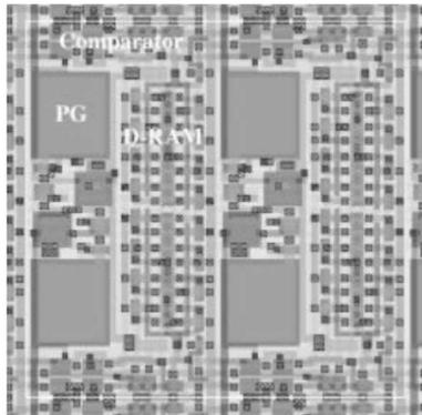
Fig. 5. DPS pixel layout (2 × 2 pixel block shown). Pixel size is 9.4 × 9.4 μm.
